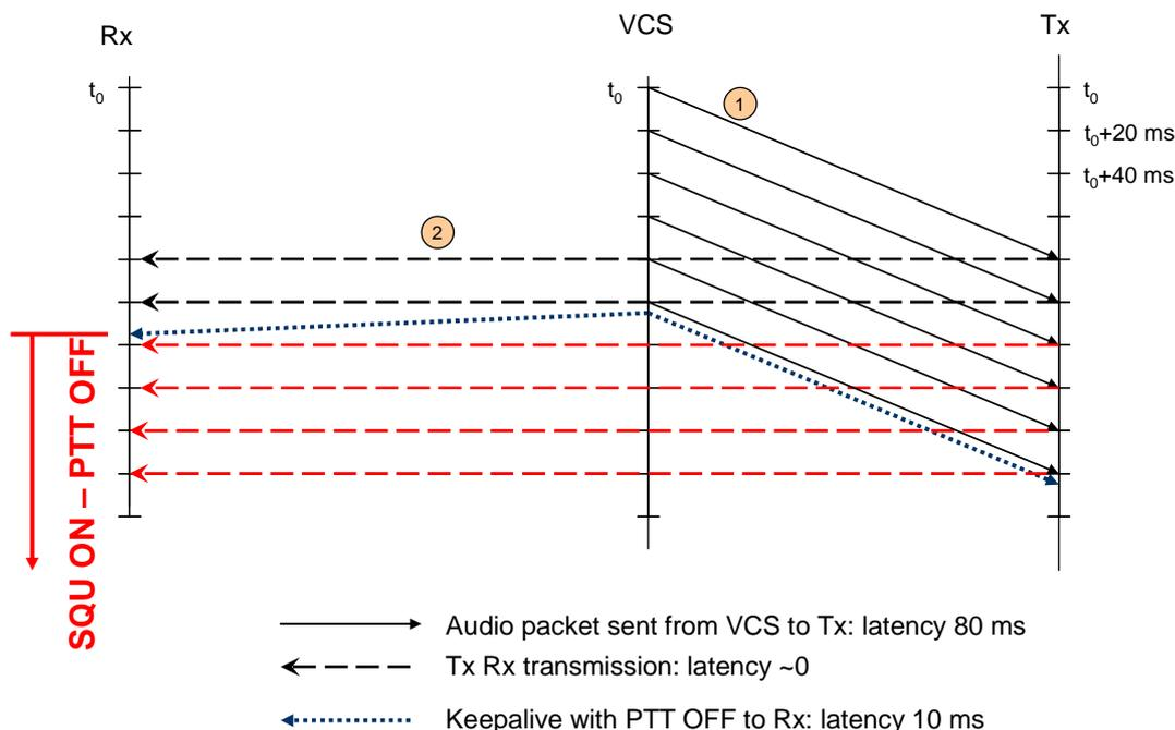
Figure 6: latency effect on separated GRS
