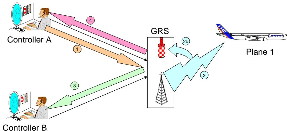
**Figure 9: 2 controllers using a single frequency - example 2**
